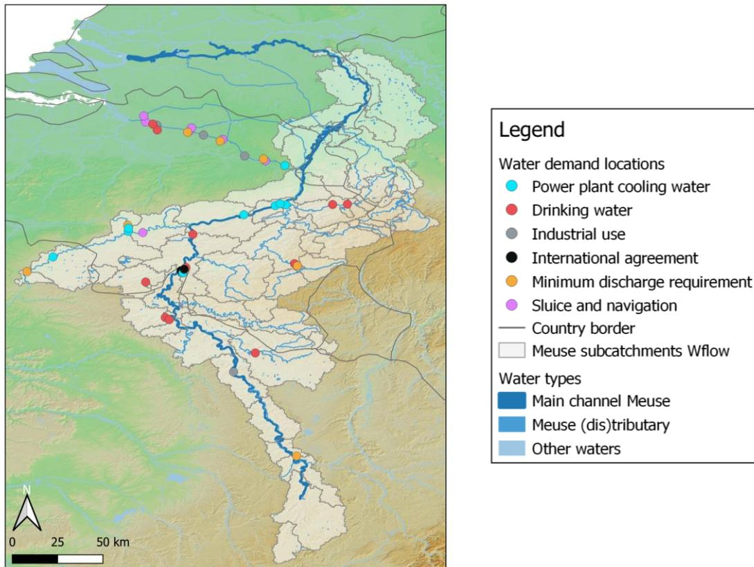
Figure 5. Sites of the water users and minimum discharge requirements in the French-Belgium Meuse catchment. The white shaded area shows the sub-catchments from the Wflow\_sbm model, used to create input time series for the RIBASIM model.
