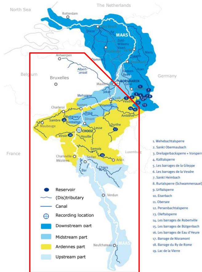
Figure 2. The Meuse catchment (Dutch: Maas) with its sub-division in four parts and the main surface water reservoirs. The red box indicates the study area of this project (adapted from Kramer, 2021).
