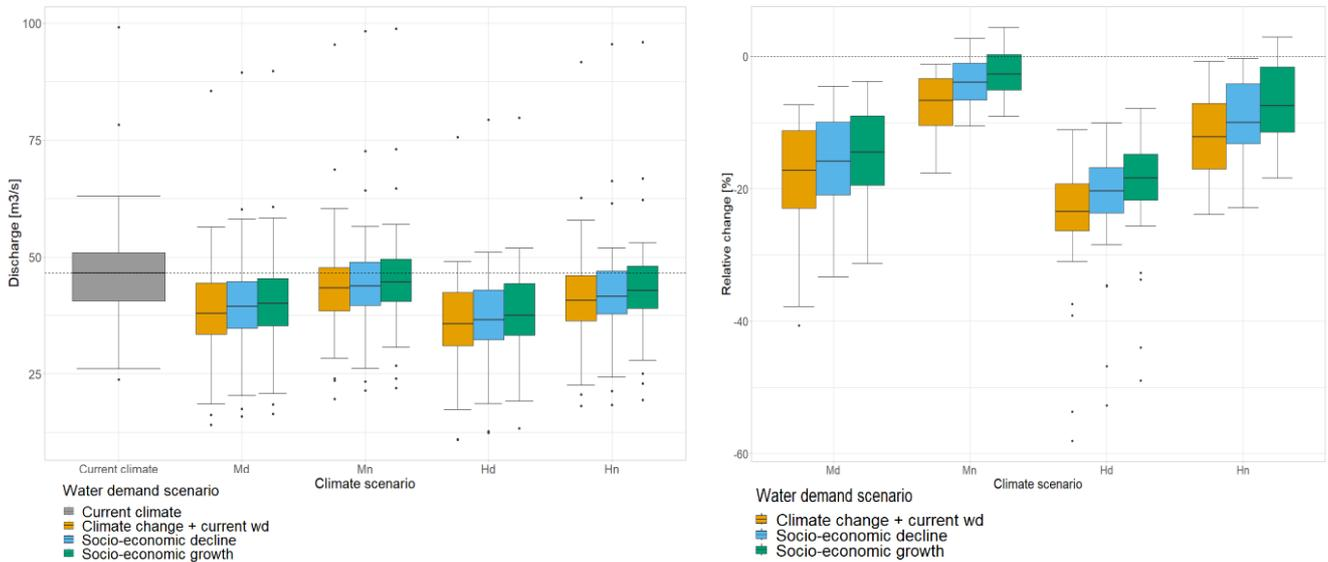
Figure 38. Change in the annual 10-day minimum discharge of the Meuse at Megen for the current climate and the moderate (Md = dry, Mn = wet) and high (Hd = dry, Hn = wet) climate scenarios for 2050, under different water demand scenarios. Left panel shows the absolute values, right panel shows the relative changes compared to the current climate (wd= water demand).
