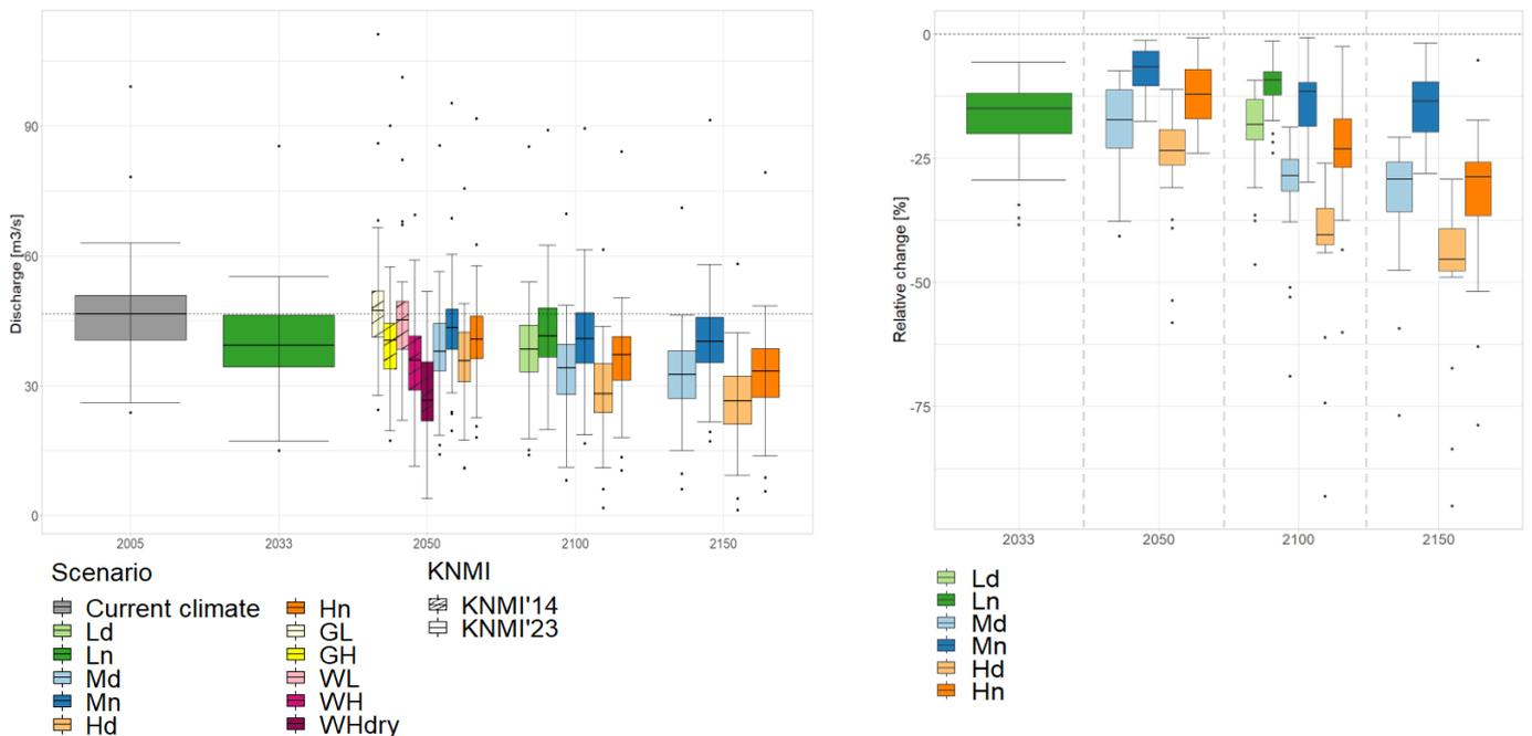
Figure 30. Change in the annual 10-day minimum discharge of the Meuse at Stenay for current and future climate (time horizons on the x axis). Left panel shows the absolute values, right panel shows the relative changes compared to the current climate for the KNMI'23 scenarios. Green boxes present the low climate change scenarios (Ln = wet and Ld= dry), blue boxes present the moderate scenarios (Mn=wet and Md=dry) and orange boxes present the high scenarios (Hn = wet and Hd =dry).
