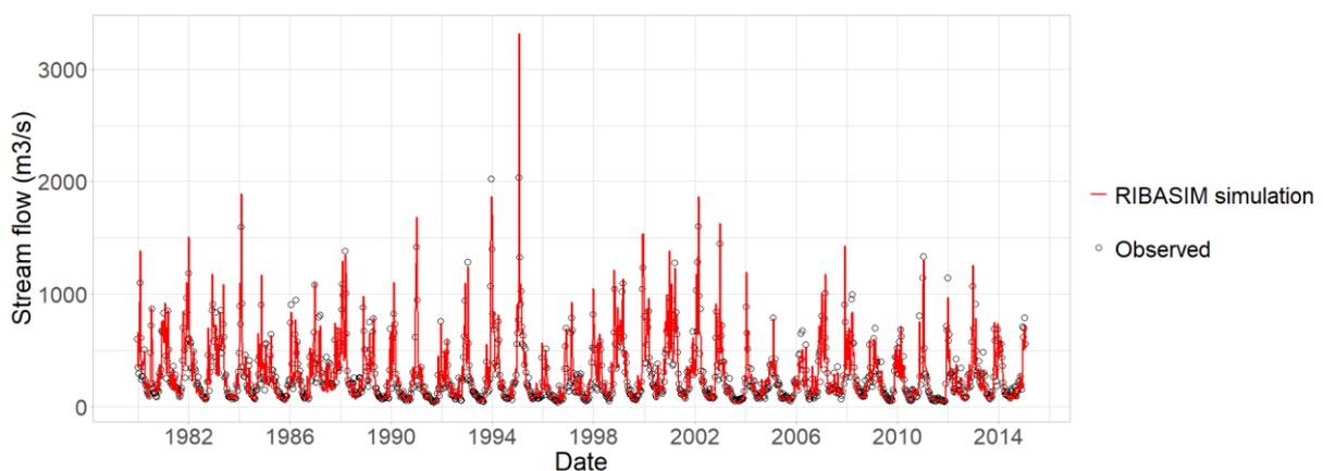
Figure 20. Discharge of the Meuse at the Flemish-Dutch border for the validation period (1980-2015). Observations in black and the RIBASIM simulation in red.
