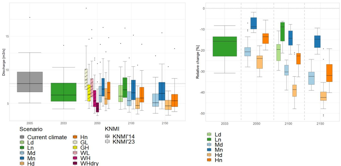
Figure 28. Change in the annual 10-day minimum discharge of the Meuse at Sedan for current and future climate (time horizons on the x axis). Left panel shows the absolute values, right panel shows the relative changes compared to the current climate for the KNMI'23 scenarios. Green boxes present the low climate change scenarios (Ln = wet and Ld = dry), blue boxes present the moderate scenarios (Mn = wet and Md = dry) and orange boxes present the high scenarios (Hn = wet and Hd = dry).
