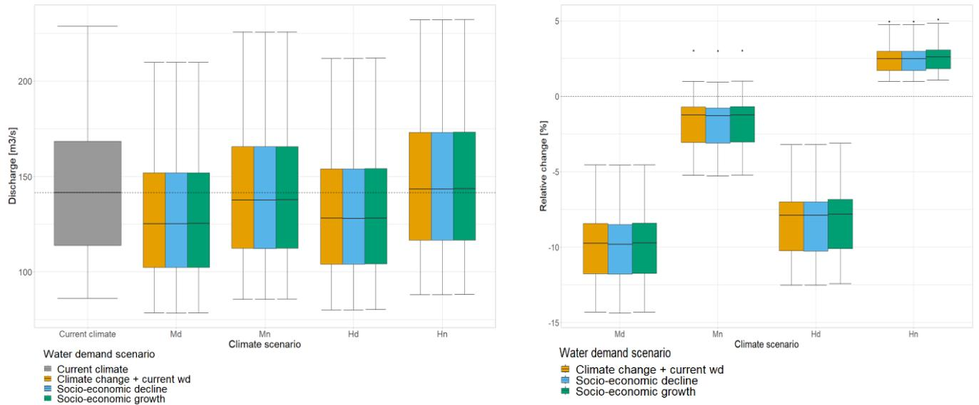
Figure 33. Change in the annual average discharge of the Meuse at Chooz for the current climate and the moderate (Md = dry, Mn = wet) and high (Hd = dry, Hn = wet) climate scenarios for 2050, under different water demand scenarios Left panel shows the absolute values, right panel shows the relative changes compared to the current climate (wd= water demand).
