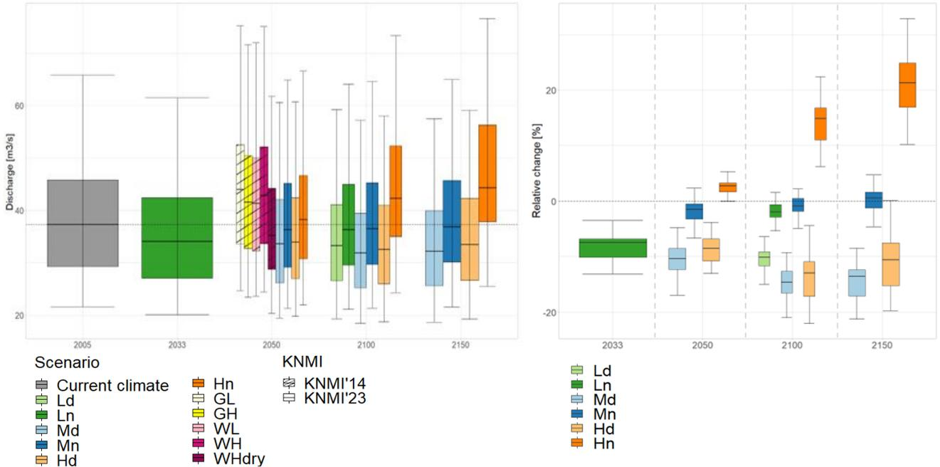
Figure 23. Change in the annual average discharge of the Meuse at Stenay for current and future climate (time horizons on the x axis). Left panel shows the absolute values, right panel shows the relative changes compared to the current climate for the KNMI'23 scenarios. Green boxes present the low climate change scenarios (Ln = wet and Ld= dry), blue boxes present the moderate scenarios (Mn=wet and Md=dry) and orange boxes present the high scenarios (Hn = wet and Hd =dry).
