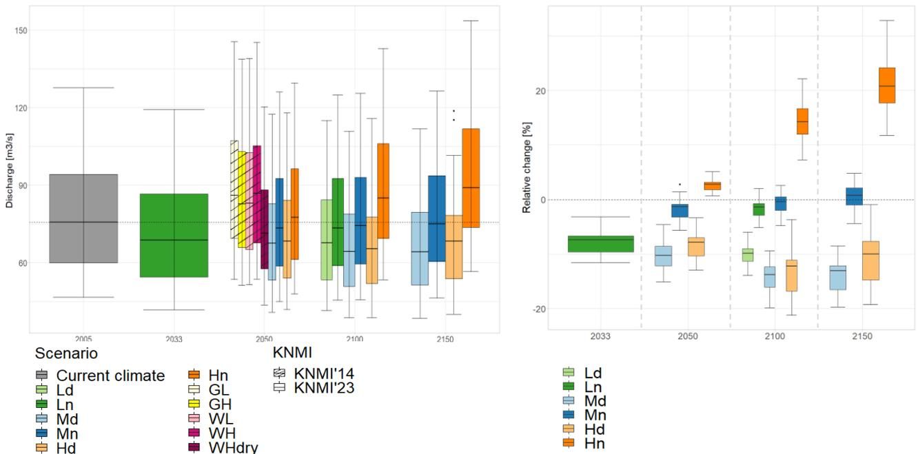
Figure 24. Change in the annual average discharge of the Meuse at Sedan for current and future climate (time horizons on the x axis). Left panel shows the absolute values, right panel shows the relative changes compared to the current climate for the KNMI'23 scenarios. Green boxes present the low climate change scenarios (Ln = wet and Ld= dry), blue boxes present the moderate scenarios (Mn=wet and Md=dry) and orange boxes present the high scenarios (Hn = wet and Hd =dry).
