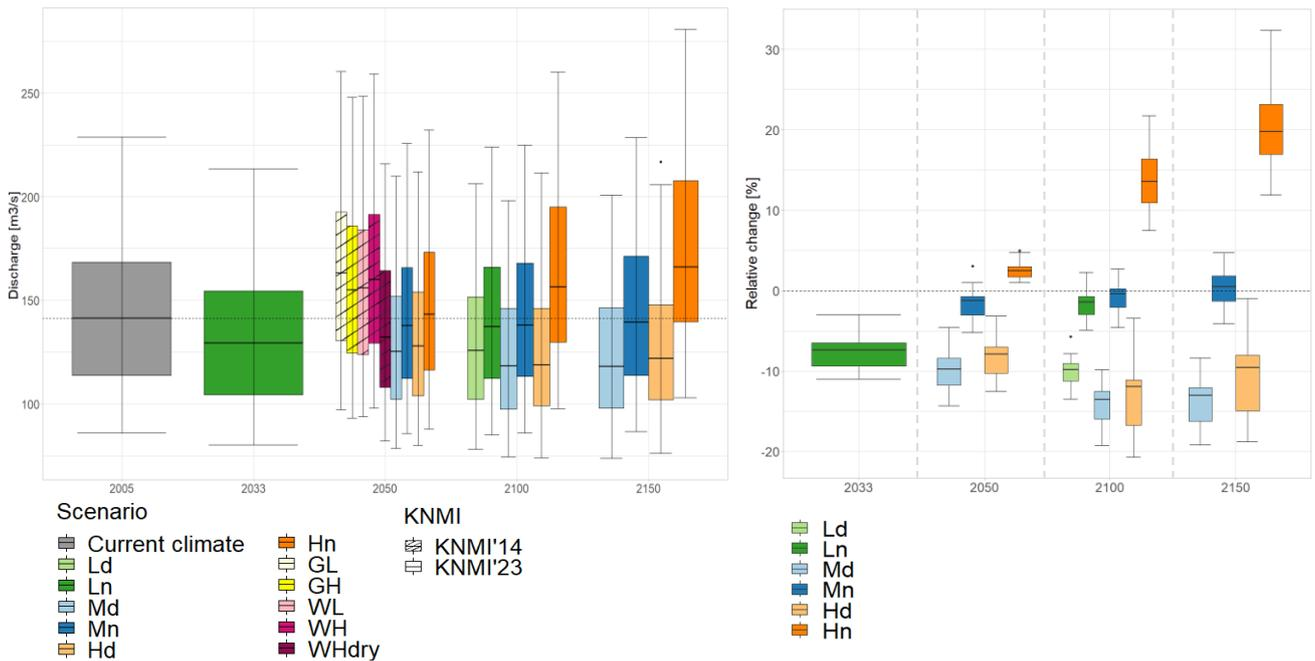
Figure 25. Change in the annual average discharge of the Meuse at Chooz for current and future climate (time horizons on the x axis). Left panel shows the absolute values, right panel shows the relative changes compared to the current climate for the KNMI'23 scenarios. Green boxes present the low climate change scenarios (Ln = wet and Ld= dry), blue boxes present the moderate scenarios (Mn=wet and Md=dry) and orange boxes present the high scenarios (Hn = wet and Hd =dry).
