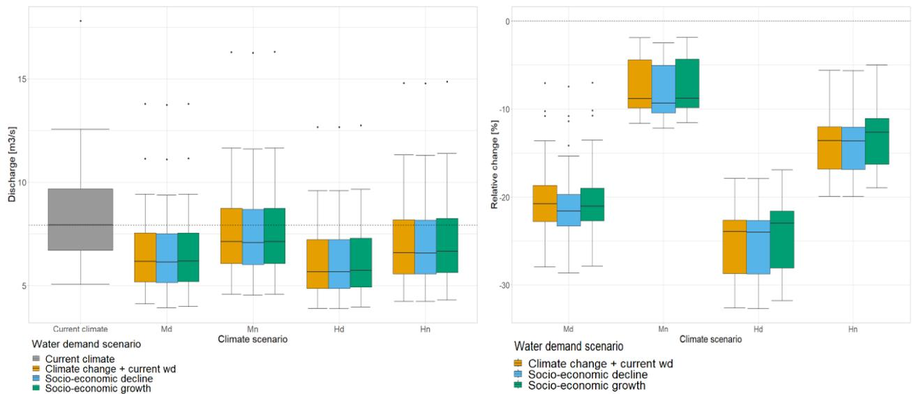
Figure 36. Change in the annual 10-day minimum discharge of the Meuse at Sedan for the current climate and the moderate (Md = dry, Mn = wet) and high (Hd = dry, Hn = wet) climate scenarios for 2050, under different water demand scenarios Left panel shows the absolute values, right panel shows the relative changes compared to the current climate (wd= water demand).
