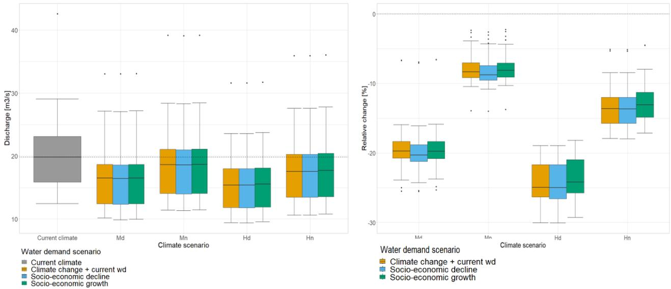
Figure 37. Change in the annual 10-day minimum discharge of the Meuse at Chooz for the current climate and the moderate (Md = dry, Mn = wet) and high (Hd = dry, Hn = wet) climate scenarios for 2050, under different water demand scenarios. Left panel shows the absolute values, right panel shows the relative changes compared to the current climate (wd= water demand).
