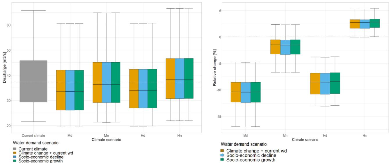
Figure 31. Change in the annual average discharge of the Meuse at Stenay for the current climate and the moderate (Md = dry, Mn = wet) and high (Hd = dry, Hn = wet) climate scenarios for 2050, under different water demand scenarios Left panel shows the absolute values, right panel shows the relative changes compared to the current climate (wd= water demand).
