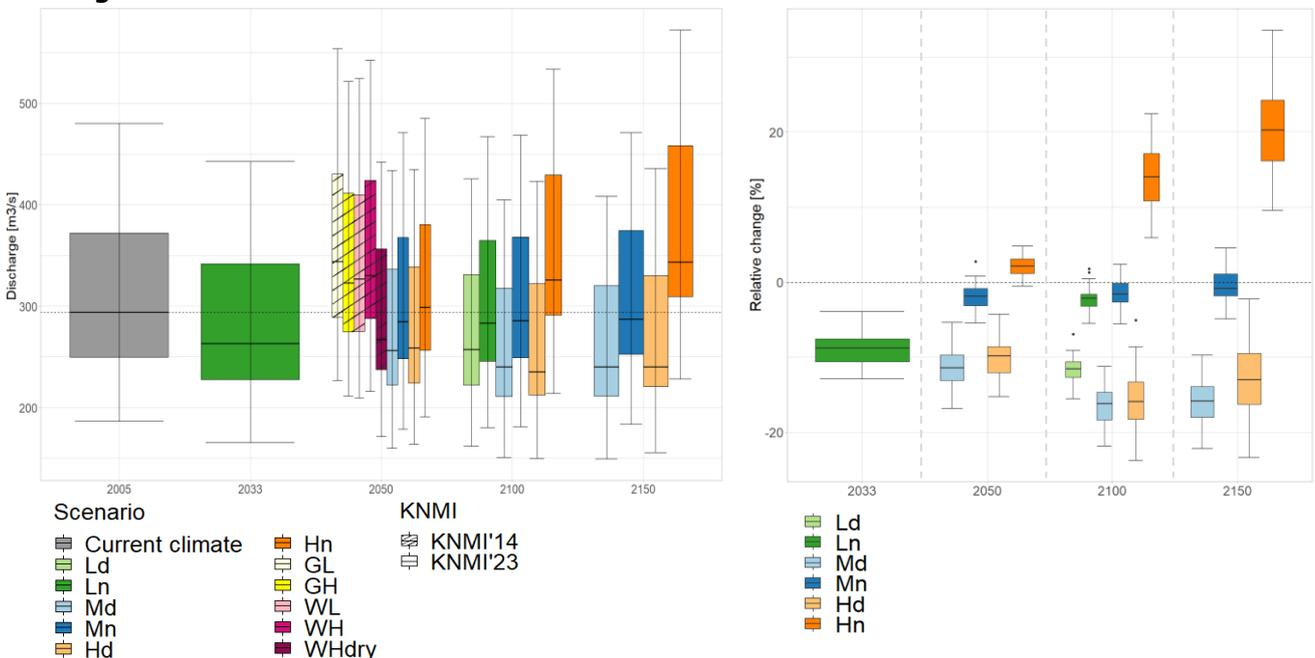
Figure 26. Change in the annual average discharge of the Meuse at Megen for current and future climate (time horizons on the x axis). Left panel shows the absolute values, right panel shows the relative changes compared to the current climate for the KNMI'23 scenarios. Green boxes present the low climate change scenarios (Ln = wet and Ld= dry), blue boxes present the moderate scenarios (Mn=wet and Md=dry) and orange boxes present the high scenarios (Hn = wet and Hd =dry).
