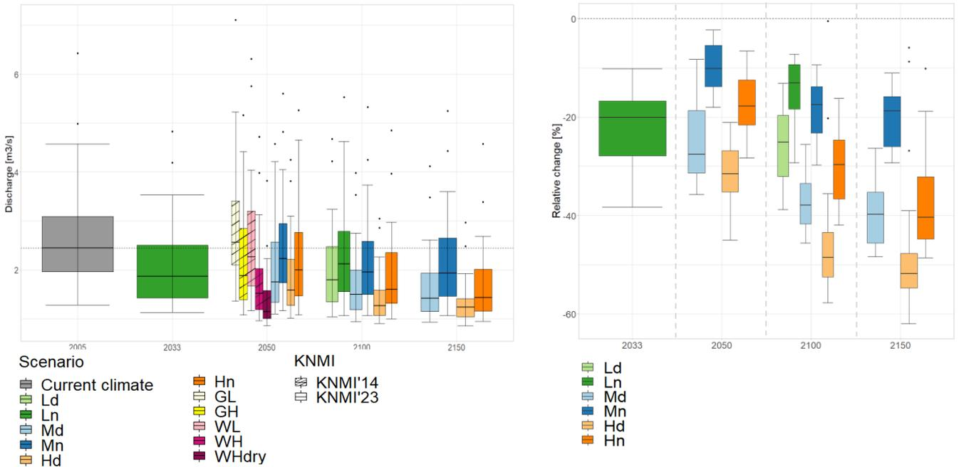
Figure 27. Change in the annual 10-day minimum discharge of the Meuse at Stenay for current and future climate (time horizons on the x axis). Left panel shows the absolute values, right panel shows the relative changes compared to the current climate for the KNMI'23 scenarios. Green boxes present the low climate change scenarios (Ln = wet and Ld = dry), blue boxes present the moderate scenarios (Mn = wet and Md = dry) and orange boxes present the high scenarios (Hn = wet and Hd = dry).
