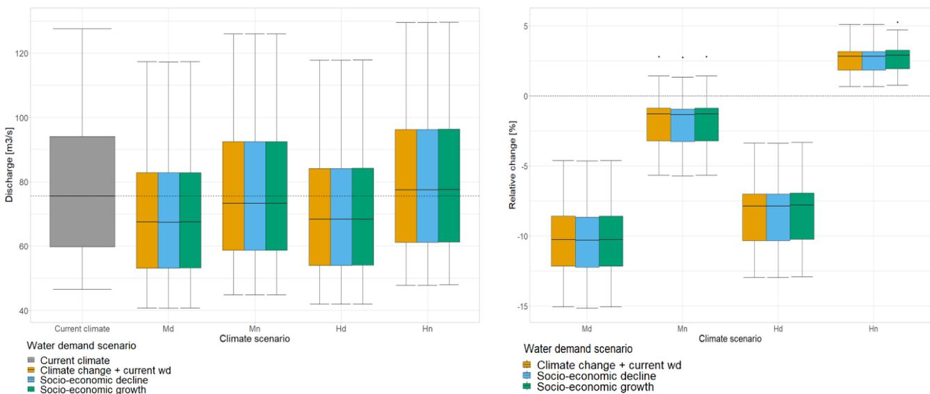
Figure 32. Change in the annual average discharge of the Meuse at Sedan for the current climate and the moderate (Md = dry, Mn = wet) and high (Hd = dry, Hn = wet) climate scenarios for 2050, under different water demand scenarios Left panel shows the absolute values, right panel shows the relative changes compared to the current climate (wd= water demand).
