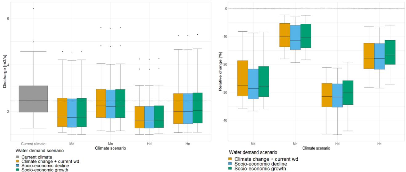
Figure 35. Change in the annual 10-day minimum discharge of the Meuse at Stenay for the current climate and the moderate (Md = dry, Mn = wet) and high (Hd = dry, Hn = wet) climate scenarios for 2050, under different water demand scenarios Left panel shows the absolute values, right panel shows the relative changes compared to the current climate (wd= water demand).
