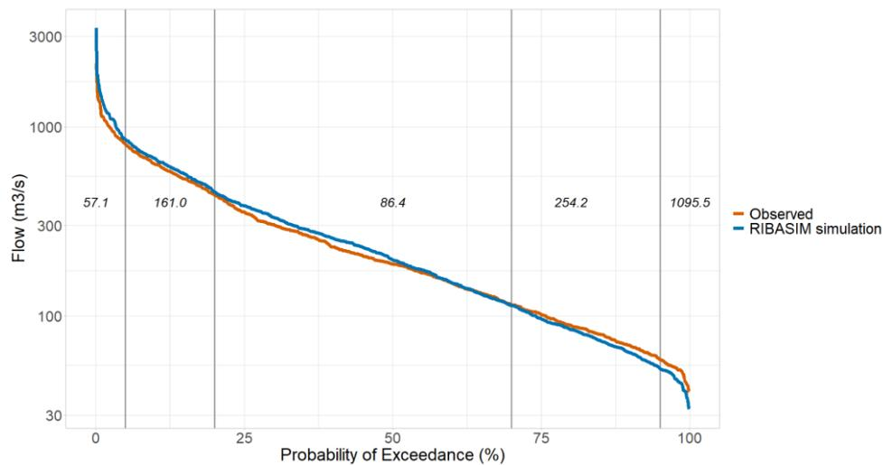
Figure 22. Flow duration curve for the observations (orange) and simulations (blue for the Meuse at the Dutch border for the period 1980-2015). The root mean square error is shown for different parts of the flow duration curve.
