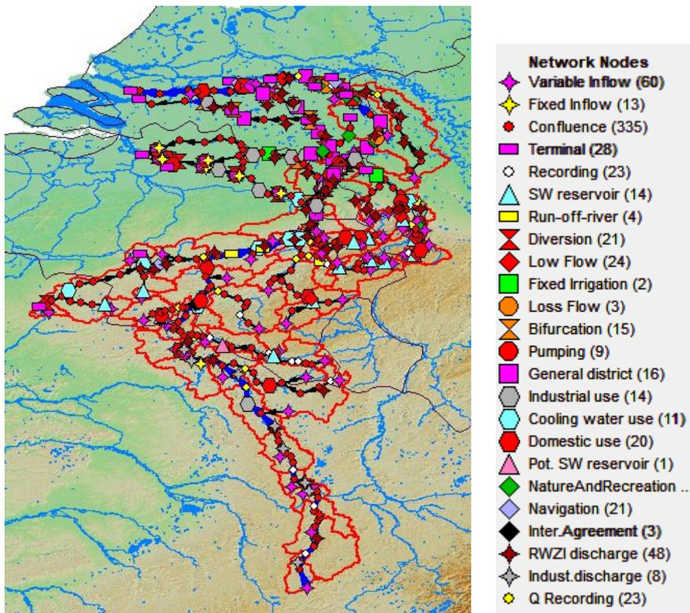
Figure 3. Network schematisation of the Meuse catchment as created by Van der Krogt et al. (2022). The black lines indicate country borders, and the red lines show the sub-catchments.
