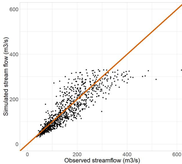
Figure 21. The relation between the observation and RIBASIM simulation of the 30% lowest discharges during the validation period (1980-2015). The orange line is the 1:1 line.
